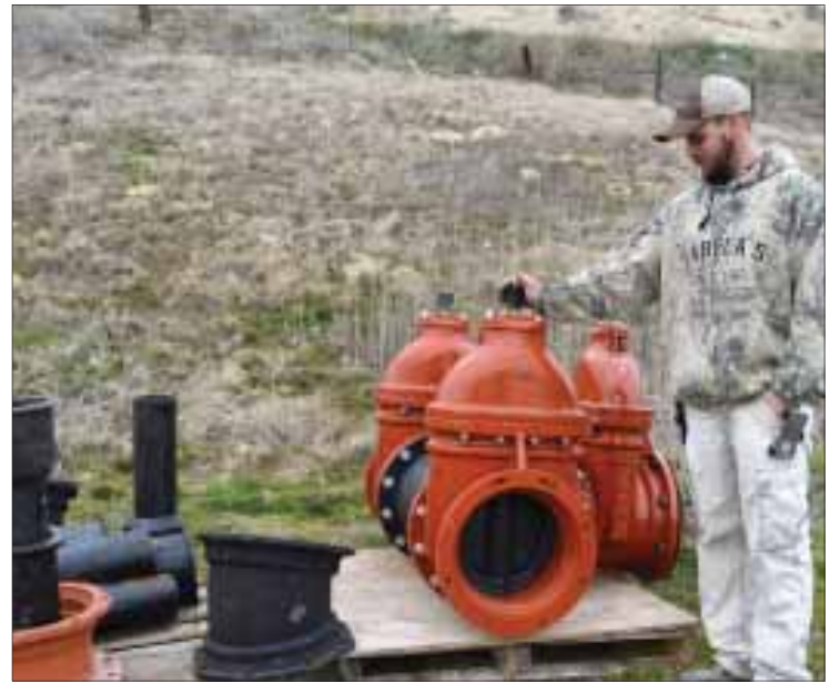
Homedale public works supervisor Bret Smith stands next to one of the gated valves prior to its installation. The valves will allow workers to isolate repairs without shutting down the entire city water system.
