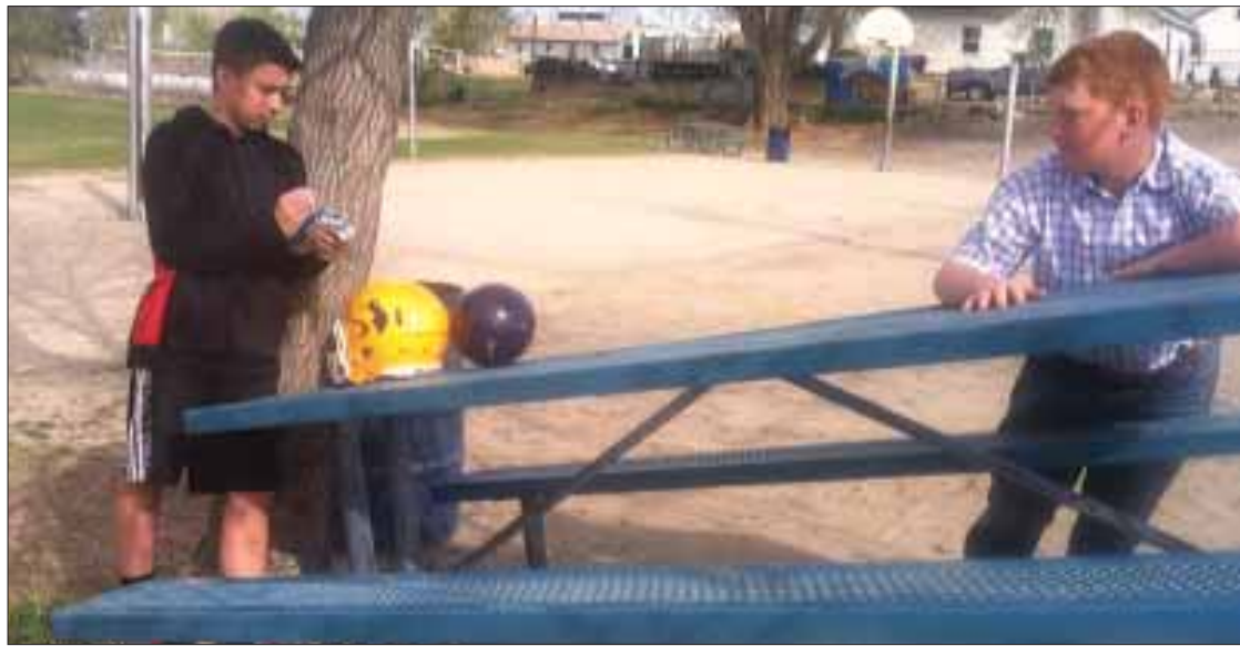
Anthony Sugai, left, and Brady Dines roll a bowling ball down an elevated picnic table to measure force impact on a Marsing High School football helmet. Submitted photo
